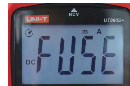
Fuse blowing alarm (mA only)
